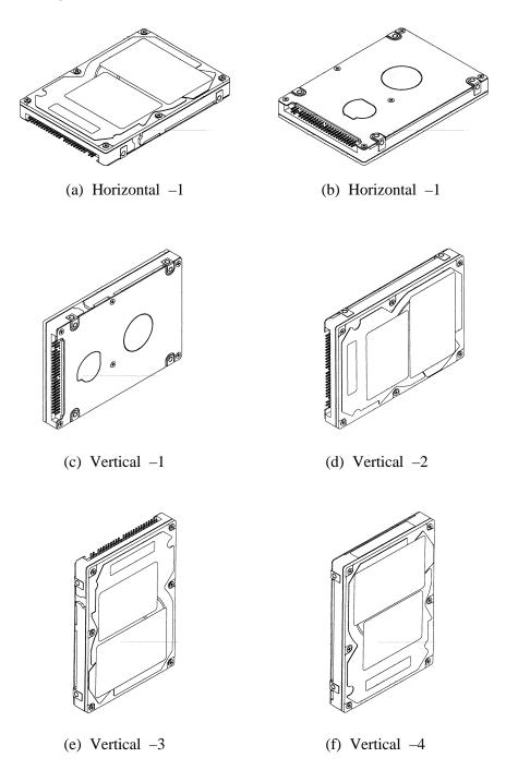
Figure 3.2 Orientation (Sample: MHC2040AT)
